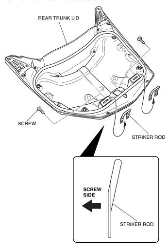
29. Remove the inner trunk lid as shown.
