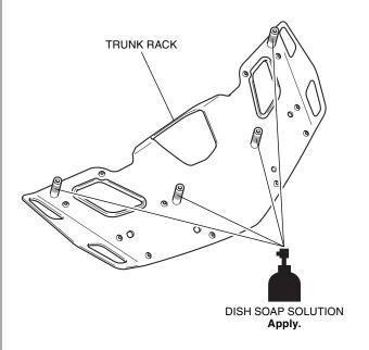
43. Install the trunk rack as shown.
