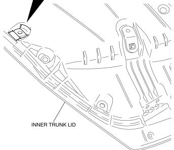
39. Install the inner trunk lid to the trunk lid as shown.
