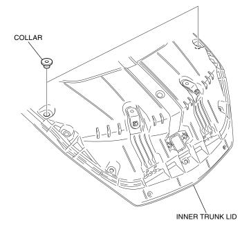
37. Clean the surface of the area shown using isopropyl alcohol.
