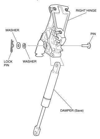
21. Remove the left trunk hinge, left hinge and damper in the same manner as the right side.
