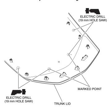
32. Install the grommets as shown.
