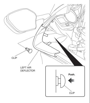
7. Pull out the adhesive backing of the left air deflector as shown.
