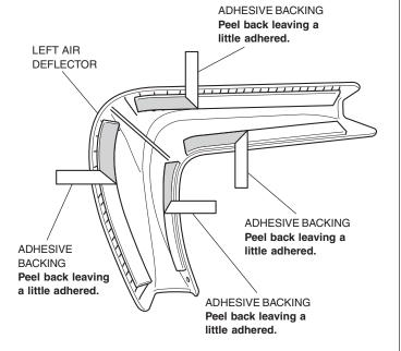
4. Clean the surface of the area shown using isopropyl alcohol.
