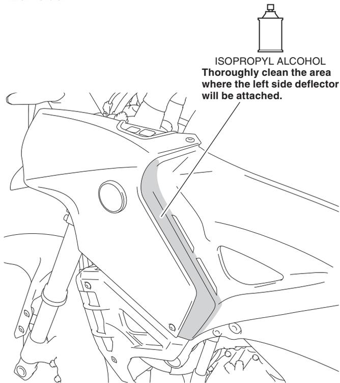
2. Peel off the adhesive backing on the rear of the left side deflector as shown.
