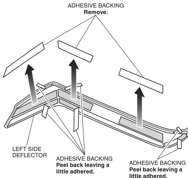
3. Attach the left side deflector by aligning it with the contour of the part it is to be attached to.
