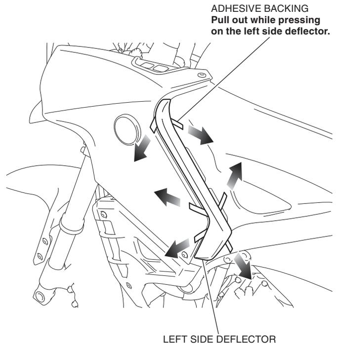
5. Apply adequate pressure to the attached left side deflector.
