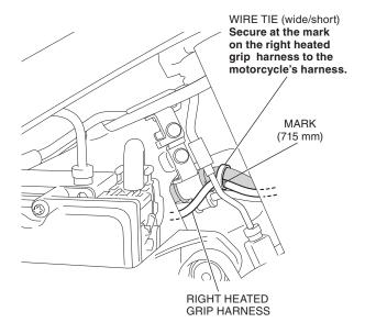
45. Secure the right heated grip harness using a wire tie as shown.
