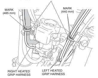
41. Secure the left heated grip harness using a wire tie as shown.
