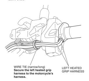
42. Secure the left heated grip harness using a wire tie as shown.
