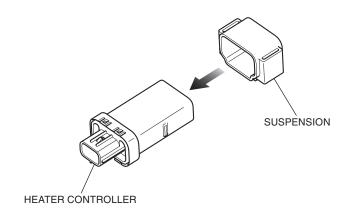
39. Connect the heater controller as shown.
