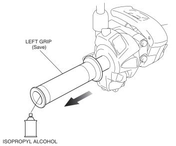
8. Using isopropyl alcohol, remove all traces of adhesive from the left handlebar pipe.
