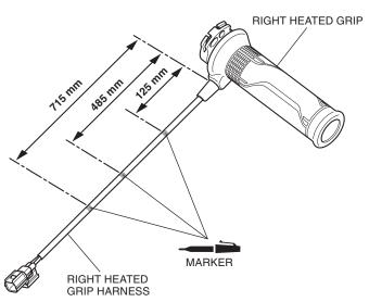
24. Wind electrical tape on the marked position as shown.
