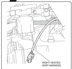
51. Secure the right heated grip harness with the clamp as shown.
