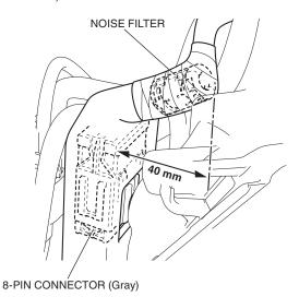
62. Remove the dummy connector as shown.
