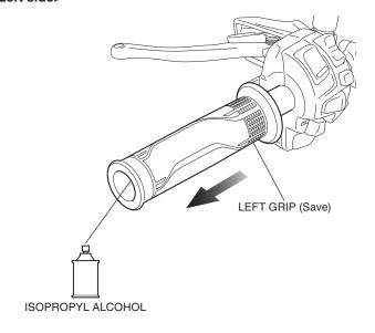
21. Using a isopropyl alcohol, remove all traces of adhesive from the left handlebar.
