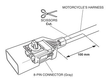
55. Take out the white wire as shown and attach electrical tape at the indicated position.
