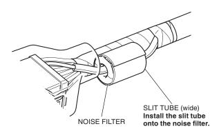
60. Secure the noise filter with electrical tape as shown.
