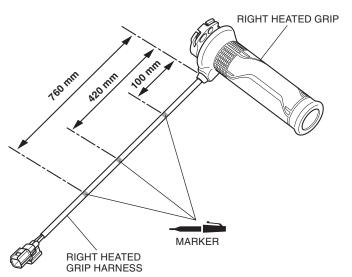
43. Install the clip bands on the marked positions as shown.
