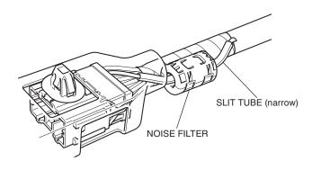
58. Wrap the slit tube with electrical tape as shown.
