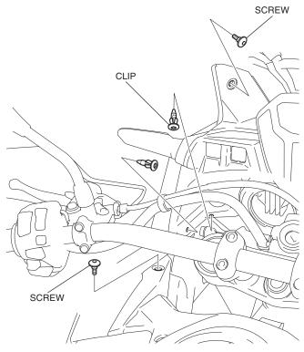
4. Remove the left tank side cover as shown.
