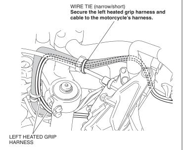
30. Secure the left heated grip harness using the wire tie as shown.
