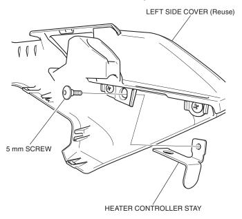
70. Install the heater controller as shown.
