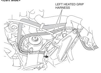
28. Secure the left heated grip harness using the wire tie as shown.
