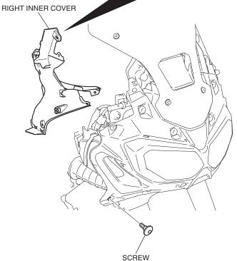
15. Remove the bolt as shown.
