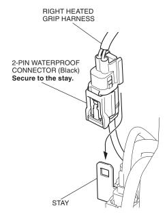
66. Secure the right heated grip harness with the wire tie as shown.
