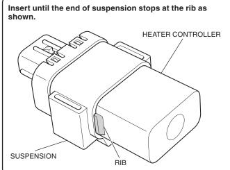
69. Install the heater controller stay as shown.
