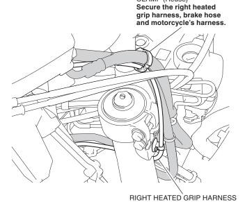
52. Remove the hose and connectors as shown. < Right side>
