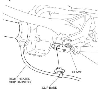
50. Route the right heated grip harness as shown and secure the harness.
