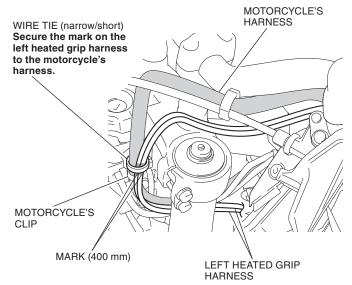
29. Secure the left heated grip harness using the wire tie as shown.
