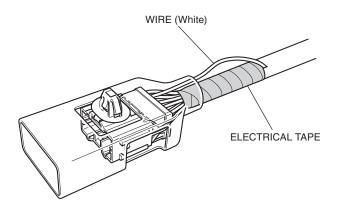
56. Install the slit tube as shown.
