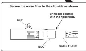
61. Install the 8-pin connector in the reverse order of removal. Make sure that the end of the 8-pin connector is within 40 mm from the end of the noise filter, as shown.
