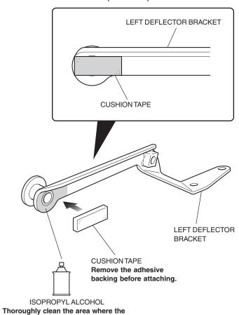
6. Loosely install the left deflector bracket as shown.
