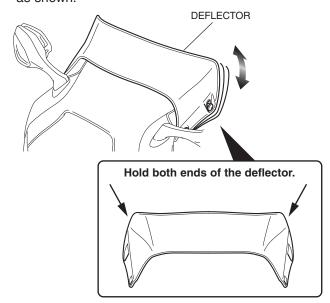
3. Tighten the left and the right screw as shown.
