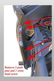
2. Remove one screw as show in picture. This will allow you to remove the inner panel.
