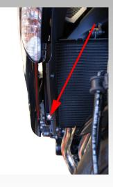
4. Fit the radiator guard if position using 2 x M6 x 12mm screws and washers provided see picture
