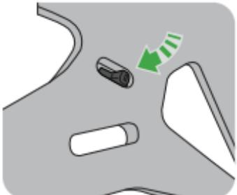
Feed cable tie through tail tidy so the head sits inside the slot on the outer face
