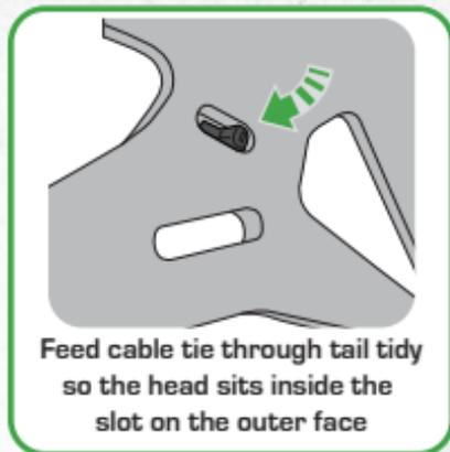
Feed cable tie through tail tidy so the head sits inside the slot on the outer face
