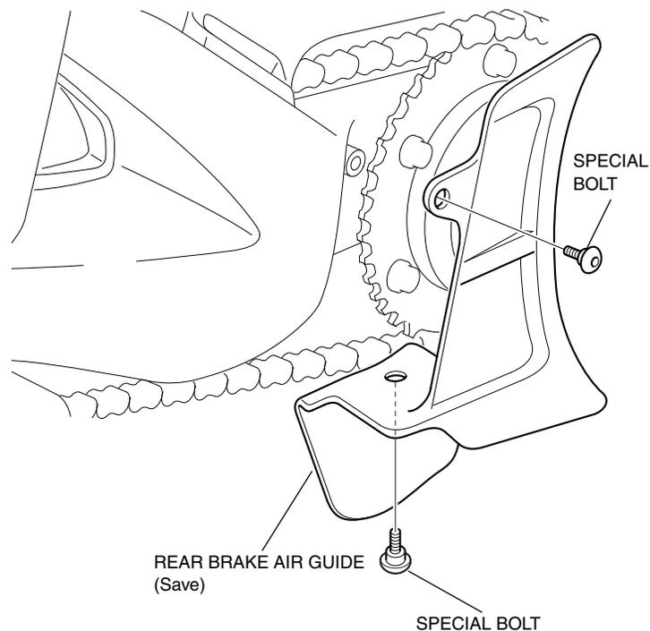
2. Apply thread lock to the mounting bolts as shown.
