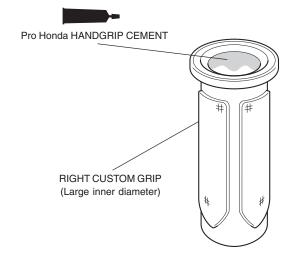
6. Apply Pro Honda Handgrip Cement to the throttle pipe and spread it with a finger as shown.
