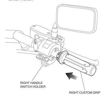
11. After installing the right custom grip on the motorcycle, check that the throttle opens smoothly and snaps shut from any opening, in any handlebar position.
