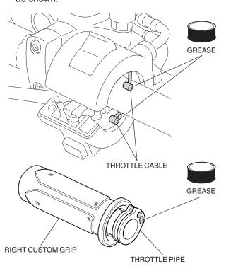
Install the right custom grip in the reverse order of original grip removal, and then install the right handle switch holder.
