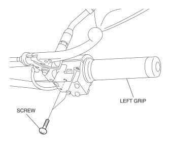
13. Remove the left handle switch holder as shown.
