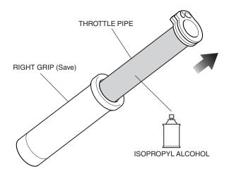
4. Use isopropyl alcohol as shown to remove any adhesive adhering to the throttle pipe.
