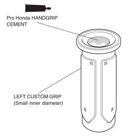
18. Apply Pro Honda Handgrip Cement to the left handlebar as shown.
