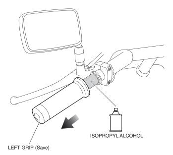
15. Use isopropyl alcohol as shown to remove any adhesive adhering to the left handlebar.
