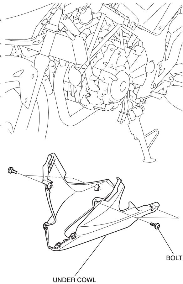
4. Disassemble the existing under cowl as shown.
