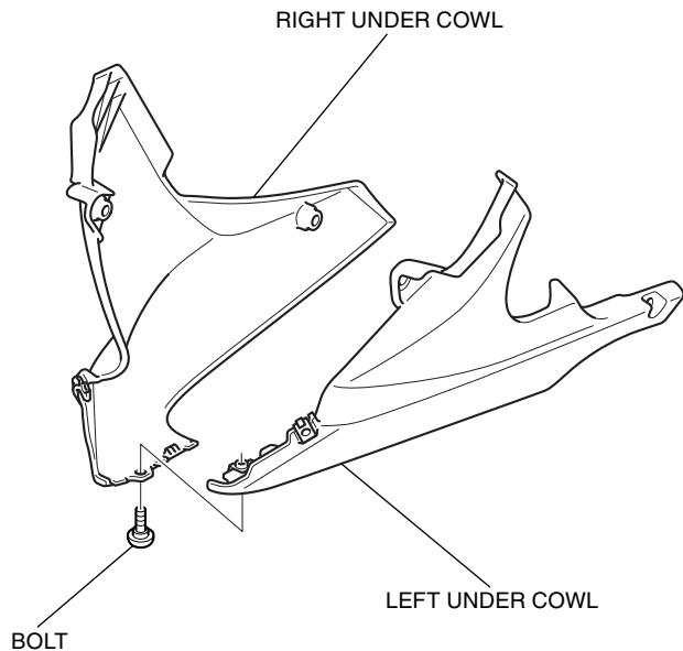
5. Replace the existing under cowl with the accessory parts as shown.
