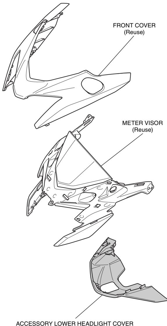
7. Install the front headlight cover in the reverse order of removal.
