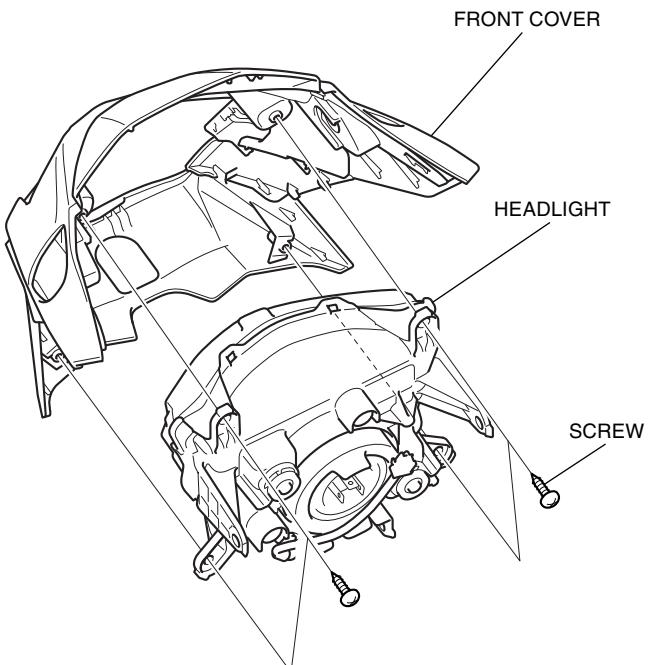
6. Replace the existing front headlight cover with the accessory cover as shown.
