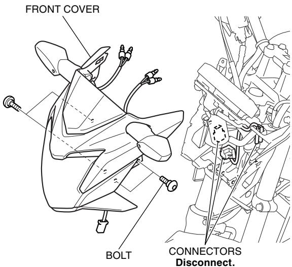
4. Remove the turn signal light as shown.
