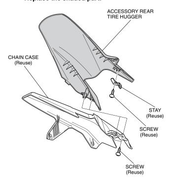
Install the removed parts in the reverse order of removal.
