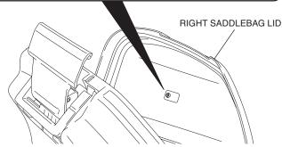
2. Peel back an end of the adhesive backings on the back of the right saddlebag panel as shown.
