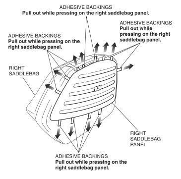
5. Apply adequate pressure to the attached right saddlebag panel.
