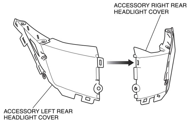
11. Install the accessory rear headlight covers in the reverse order of removal.
