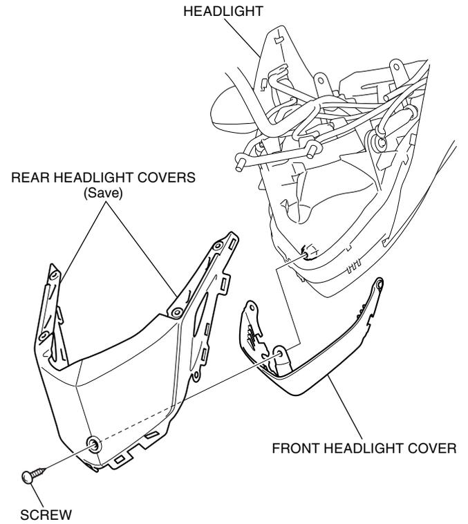
10. Assemble the accessory rear headlight covers as shown.
