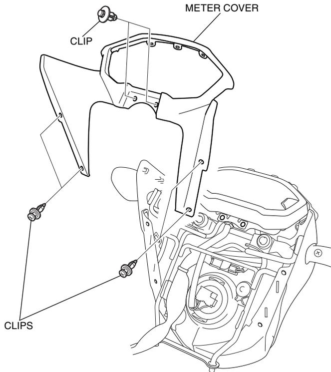
8. Refer to the Service Manual for the motorcycle, remove the meter visor.
