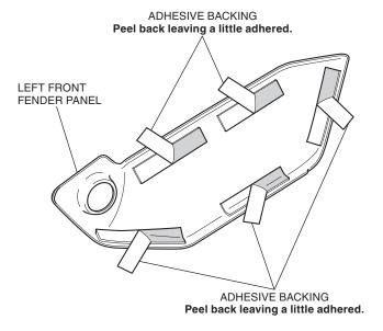
4. Attach the left front fender panel as shown.
