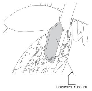
3. Peel off the adhesive backing on the left front fender panel as shown.
