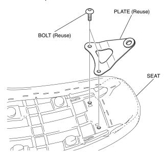
7. Remove the bolts, belt, and stay from the seat as shown.
