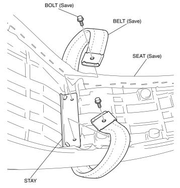
8. Install the stay, accessory belt, and bolts in the reverse order of removal.
