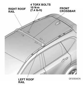
4. Position the rear crossbar onto the left and right roof rails. Install the rear crossbar the same way.
