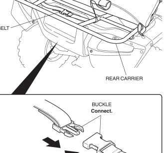
2. Position the rear rack bag on the rear carrier and secure it by tightening the belt as shown.
