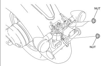
8. Remove the rear turn signal light as shown.
