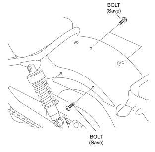
Install the 8 mm bolts and rear carrier as shown.
