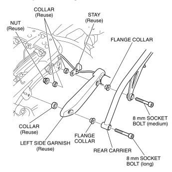
6. Install the removed parts in the reverse order of removal.
