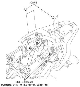
8. Install the motorcycle's parts in the reverse order of removal.
