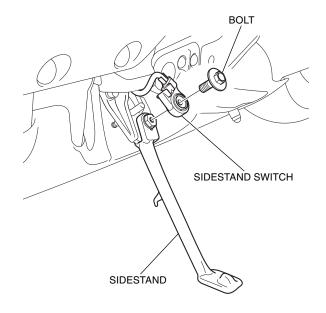
3. Remove the pivot bolt and sidestand as shown.
