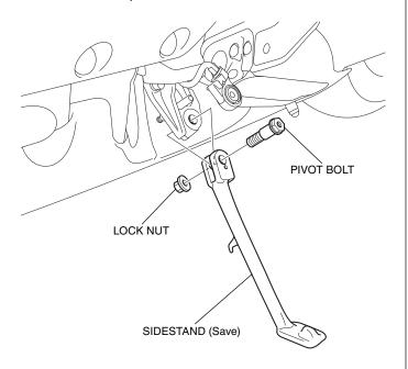
4. Apply grease to the accessory sidestand in the positions shown.
