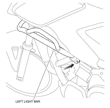
14. Loosely install the 6 mm flange bolts and nuts as shown.
