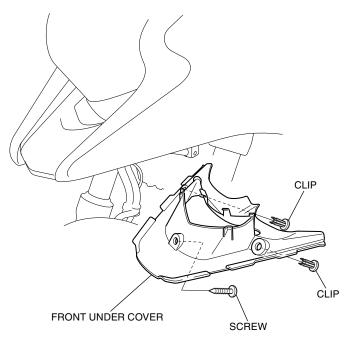
6. Cut and attach the template to the front under cover and mark it using a marker as shown.
