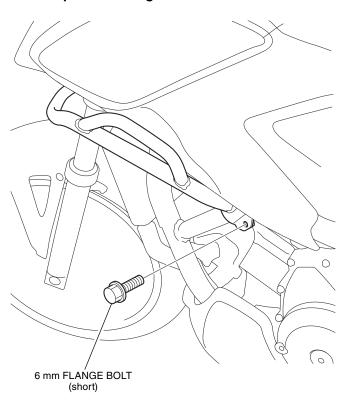
16. Tighten all loosely installed hardware to the specifications in the torque chart.
