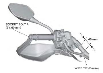
7. Perform the following for NC700XD model only: Install the cable clip to the right handguard stay as shown.
