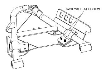
4. Thread a U-nut onto each screw and tighten until the bracket loosely contacts the guard.
