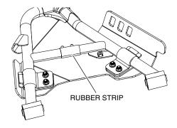
7. Assemble the bracket over the rubber strip as shown.
