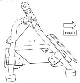
3. Pass two screws through the countersunk holes in the guard and assembled bracket as shown.
