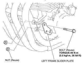
3. Install the engine guard base as shown.
