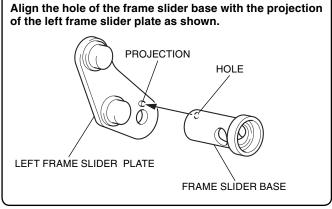
4. Install the frame slider body as shown.
