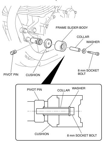
5. Install the frame slider cap as shown.
