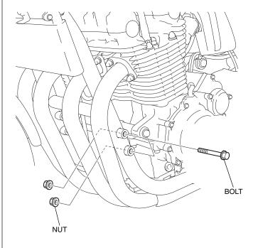
2. Install the left frame slider plate as shown.
