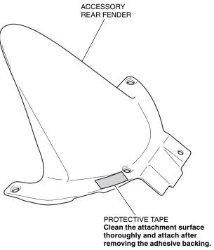
3. Install the accessory rear fender in the reverse order of removal.
