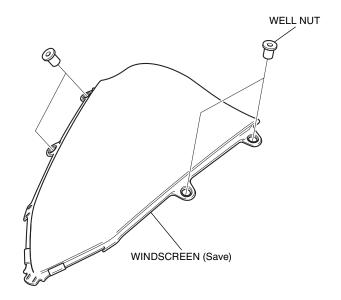
13. Install the well nuts as shown.
