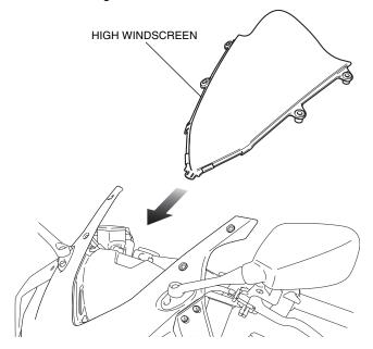
15. Install the parts as shown.
