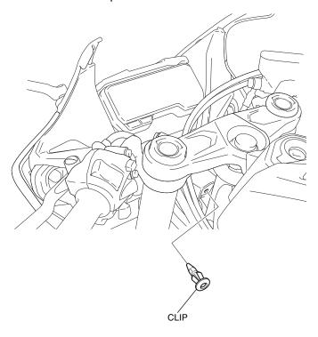
6. Remove the meter as shown.
