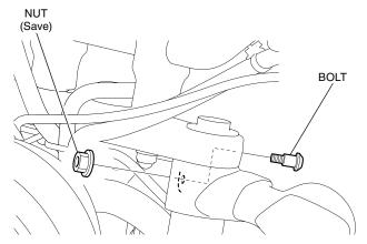
3. Loosely install the meter visor stay as shown.
