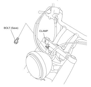
3. Install the assembled screen stay as shown.
