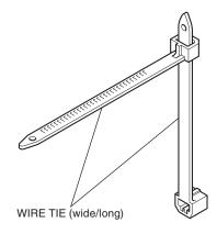
55. Secure the heated grip harness and boot cover with the wire ties as shown.
