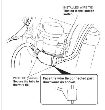
48. Secure the heated grip harness and left heated grip harness with the wire tie as shown.
