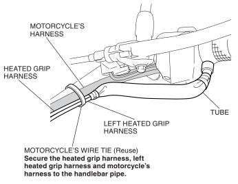
49. Secure the tube with the wire tie as shown.
