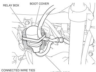
CONNECTED WIRE TIES Secure the heated grip harness and boot cover to the relay box.
