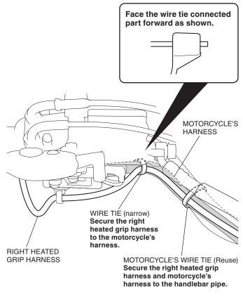
51. Secure the heated grip harness with the wire ties as shown.
