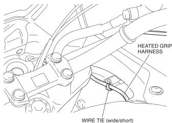
WIRE TIE (wide/short) Secure the heated grip harness to the right shroud.
