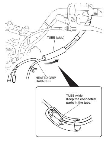
39. Pass the grip heater harness through the tube as shown.
