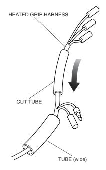
34. Connect the heated grip harness as shown. <Left side>
