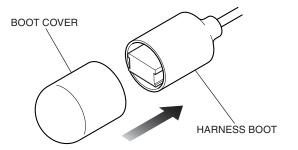
31. Secure the boot cover with electrical tape as shown.
