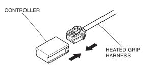
29. Fit the harness boot over the controller as shown.
