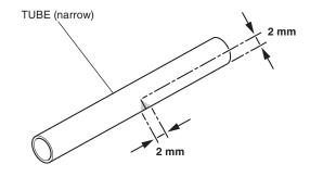
33. Pass the tube and cut tube over the heated grip harness as shown.
