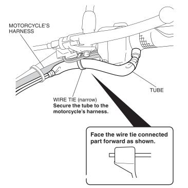
50. Secure the right heated grip harness with the wire ties as shown.
