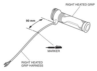
11. Install the clip band on the marked position as shown.
