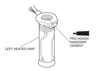
22. Apply Pro Honda Handgrip Cement to the left handlebar as shown.
