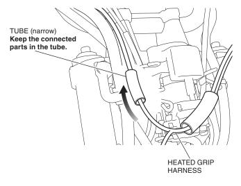
42. Secure the tube with electrical tape as shown.
