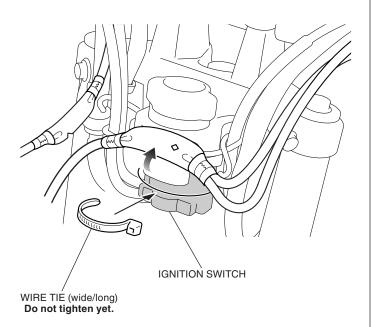
47. Secure the tube with the wire ties as shown.
