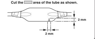
44. Secure the tube with electrical tape as shown.
