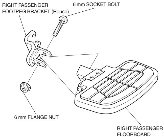
4. Install the right passenger floorboard as shown.
