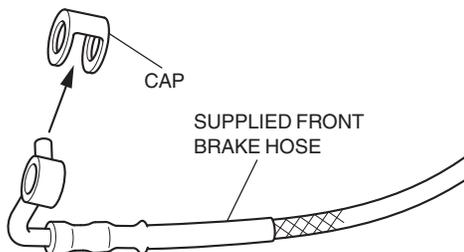
9. Install the supplied front brake hose in the reverse order of the original hose removal.
