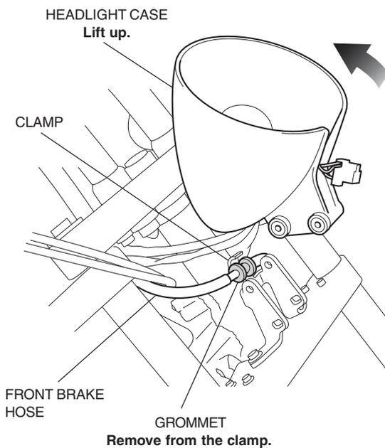
6. Disengage the front brake hose grommet from the clamp as shown.
