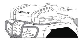
2. Identify the tubes that the bag will anchor to on the front rack. Ensure that all hook and loop straps will reach a secure position on the rack.
