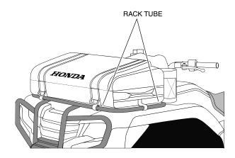
Secure each hook and loop strap around the rack tube
