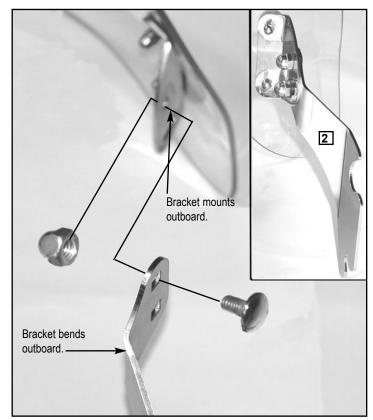
Figure 2. Right Side Bracket Assembly
