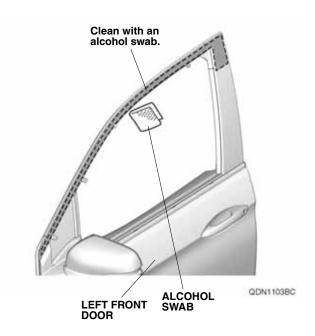
7. Attach a piece of masking tapes to the end of the adhesive backings as shown. Peel back the adhesive backings partway and temporarily attach them to the front surface of the left front door visor.
