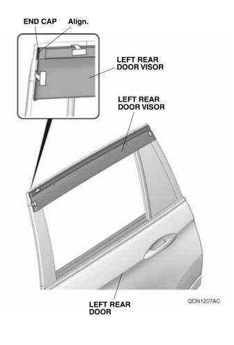
22. While applying light pressure against the left rear door visor, carefully remove the taped adhesive backings. Make sure to push up on the two brackets A while removing the adhesive backings. NOTE: While removing long top piece of adhesive backing, make sure that left rear door visor is positioned so that top edge of vehicle chrome is hidden by left rear door visor.
