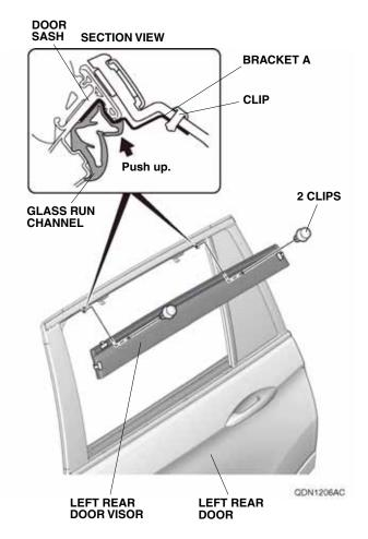
20. Secure the left rear door visor to two brackets A with two clips. Make sure to push up on the two brackets A while installing two clips. NOTE: The clips cannot be removed and reinstalled after installation. 21. Align the left rear door visor as shown.
