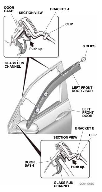
9. Secure the left front door visor to two brackets A and one bracket B with three clips. Make sure to push up on the two brackets A and one bracket B while installing the clips.
