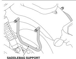
• Check the accessory mounts frequently and retighten if necessary.
