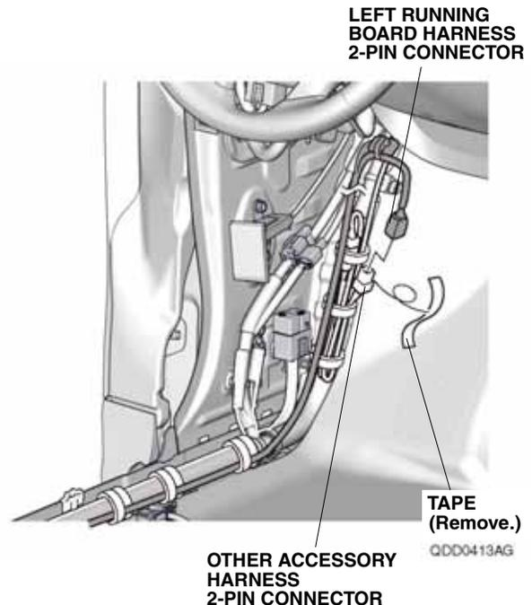
26. Bundle up the excess left running board harness, and secure it to the vehicle harness with two wire ties. Go to step 30.
