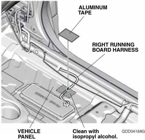
34. Secure the right running board harness to the vehicle panel with one aluminum tape as shown.
