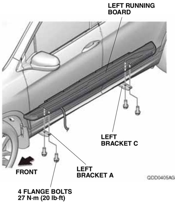
13. Tighten the four flange bolts loosely installed in step 11. Torque the flange bolts to 27 N·m (20 lb·ft).
