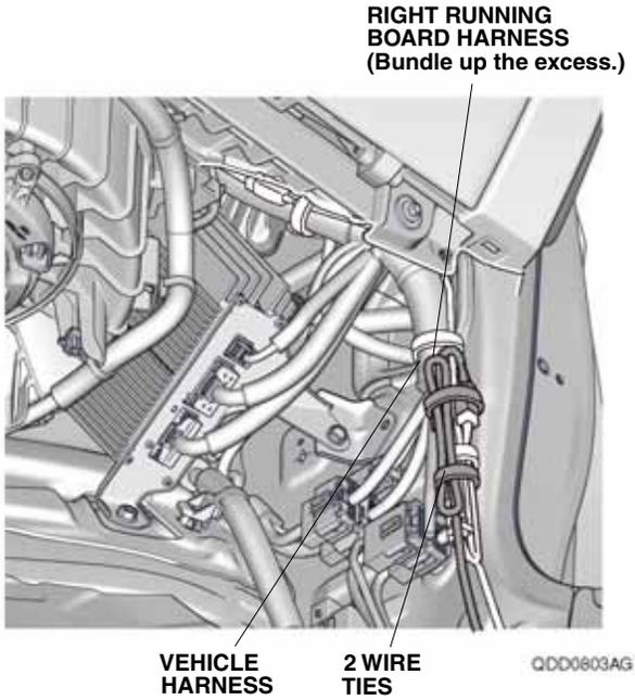
40. Secure the right running board harness to the vehicle harness with two wire ties.
