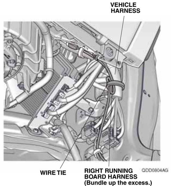
42. Check that all wire harnesses are routed properly and all connectors are plugged in.
