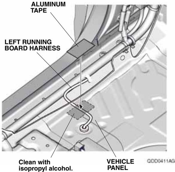
22. Secure the left running board harness to the vehicle panel with one aluminum tape as shown.
