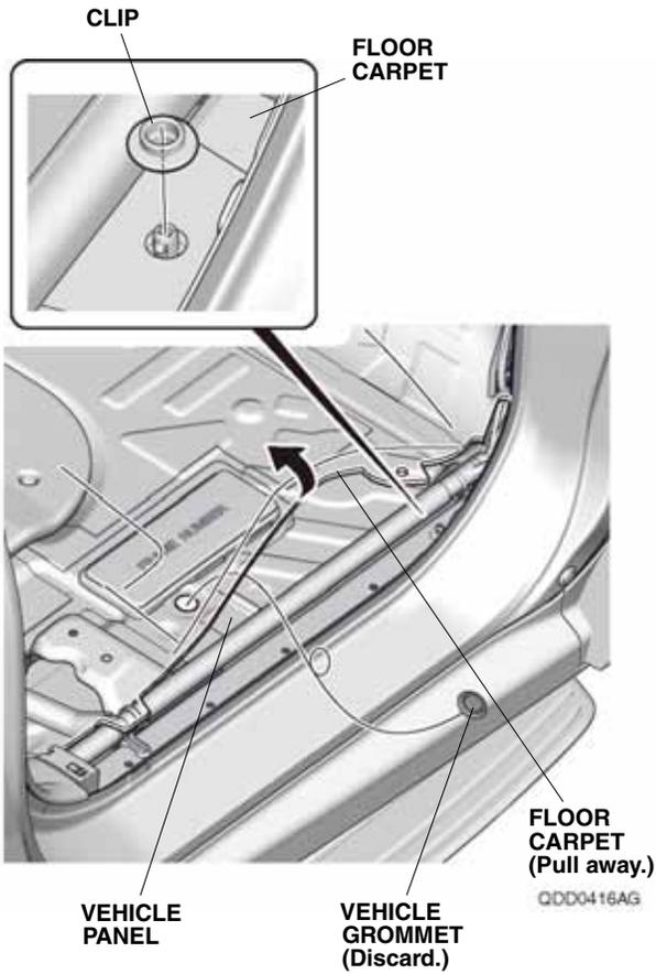
31. Locate the vehicle grommet, and remove it from the vehicle panel.
