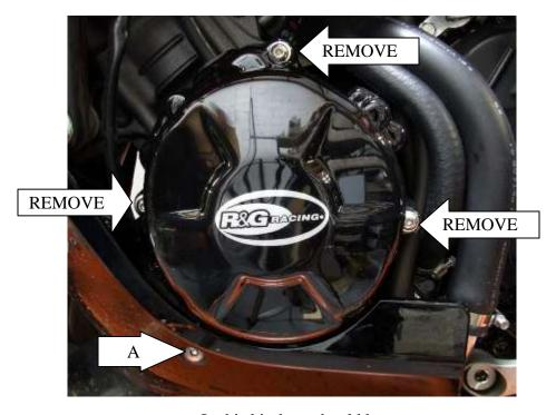
In this kit there should be 1 x Engine Case Cover (ECC0021) 3 x M6x40mm long button head bolts
