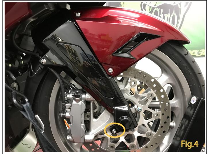
8. Install fork leg cover onto motorcycle. It may be necessary to temporarily move front fender slightly out of position.
