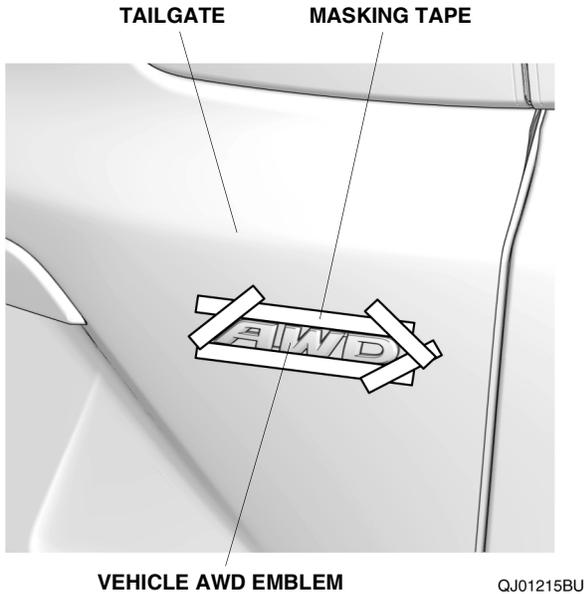
33. Using a piece of string, remove the vehicle AWD emblem by cutting along the outer edges as shown. NOTE:
