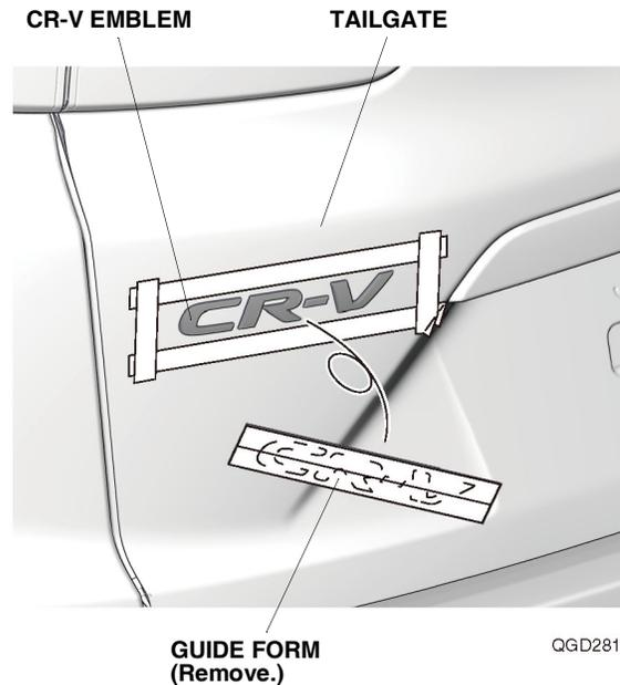
31. Remove the masking tape from the tailgate.
