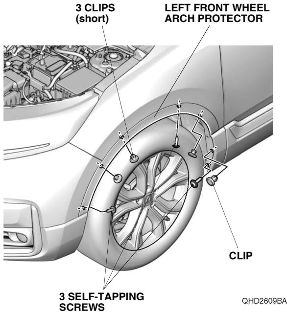
5. Remove the left front wheel arch protector as shown.
