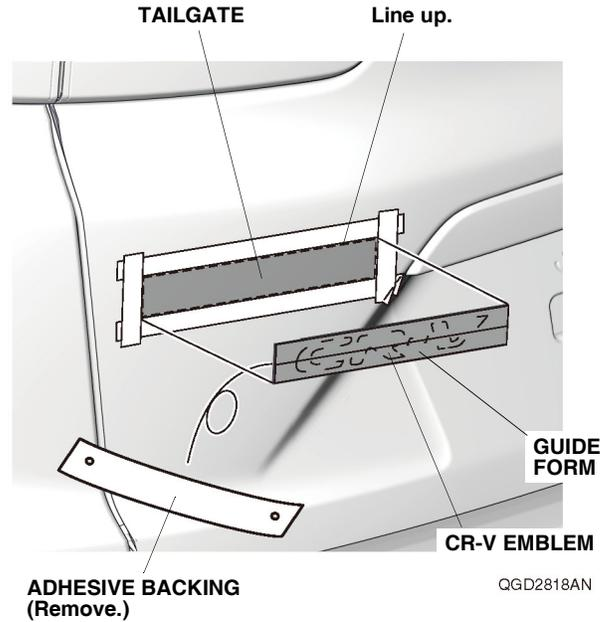
30. Remove the guide form and using the palm of your hand, firmly press the CR-V emblem against the tailgate.
