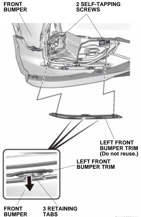
7. Install the new left front bumper trim to the front bumper with two self-tapping screws and three retaining tabs.
