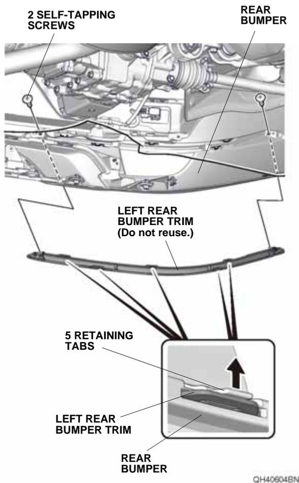
11. Install the new left rear bumper trim to the rear bumper with two self-tapping screws and five retaining tabs.
