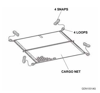
Attach four snaps from the cargo net to the cargo hooks shown.
