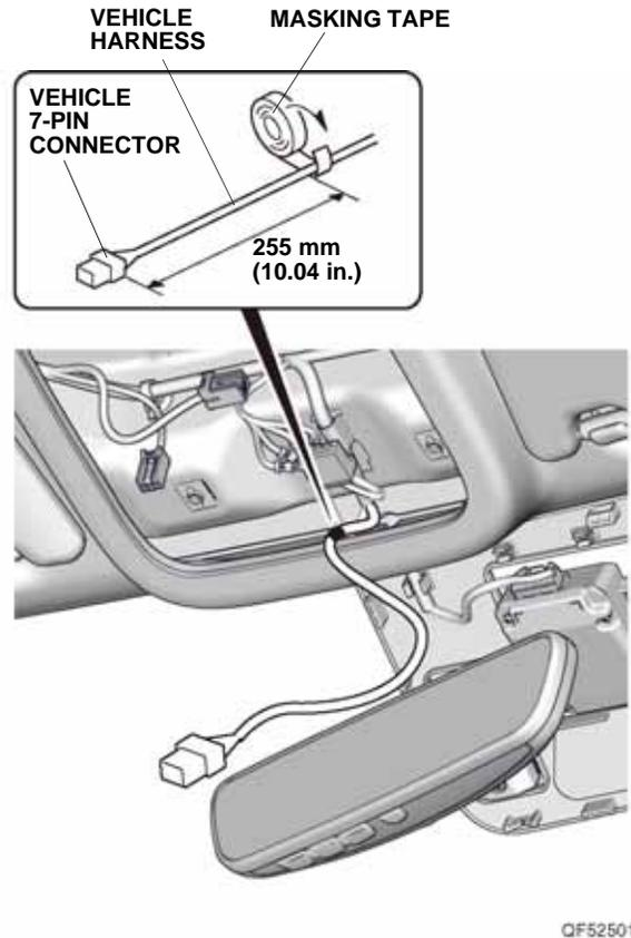
9. Route the vehicle harness as shown. Be careful not to crease the headliner. Secure the vehicle harness to the holder on the camera cover base, and plug the vehicle 7-pin connector into the automatic day/night mirror.
