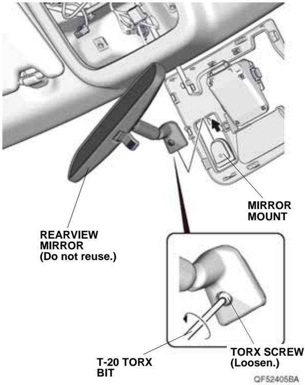
6. Install the automatic day/night mirror on the mirror mount as shown, and tighten the TORX screw.
