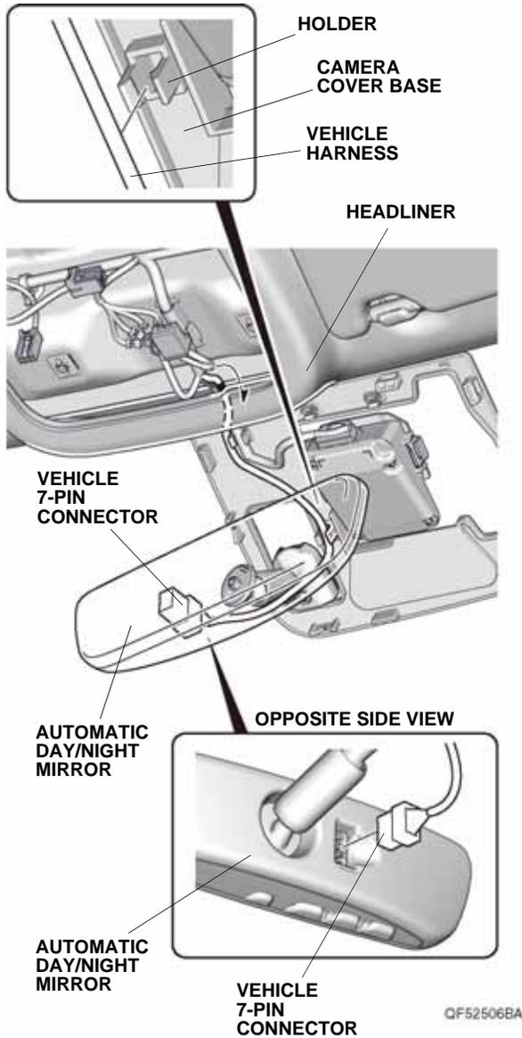
10. Using isopropyl alcohol on a shop towel, thoroughly clean the camera cover base where the aluminum tape will attach.
