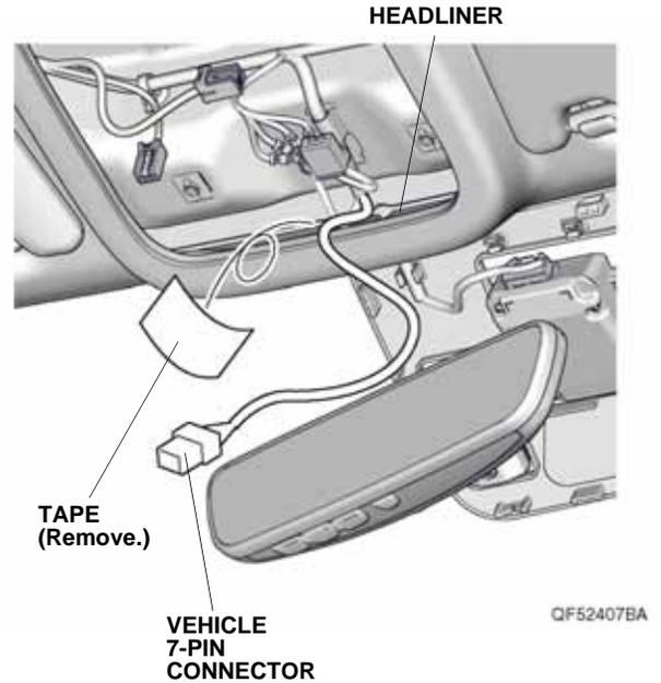
8. Attach masking tape to the vehicle harness at the measurement shown.
