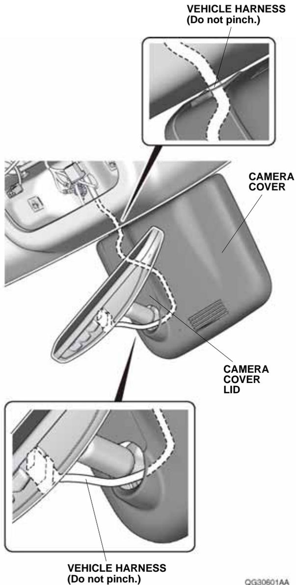
13. Check that all wire harnesses are routed properly and all connectors are plugged in.
