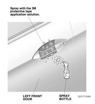
3. Remove the adhesive backing from the left front door handle film.
