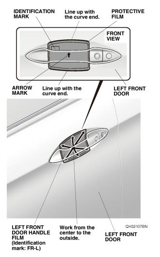
6. Starting from the center and working outward, use the mini soft spreader/applicator to smooth out the left front door handle film. If you see an air bubble, stop and gently peel up that section to work out the bubble. Work slowly and keep pressure against the left front door handle film. 7. Remove the protective film from the left front door handle film. Using a shop towel, wipe up the 3M protective tape application solution. Allow the left front door handle film to dry thoroughly.
