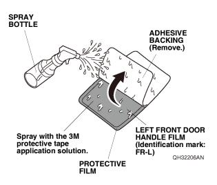
4. Spray the left front door handle film and protective film with the 3M protective tape application solution.
