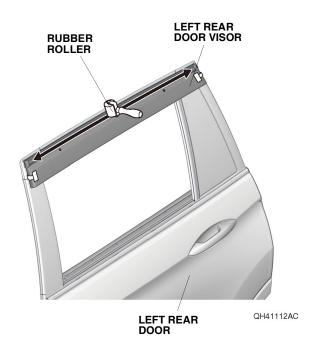
26. While applying light pressure against the left rear door visor, carefully remove the taped adhesive backings.
