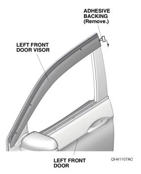
14. Using a rubber roller, apply firm pressure against the left front door visor and roll from one end to the other. NOTE: Apply firm pressure, especially at the ends.
