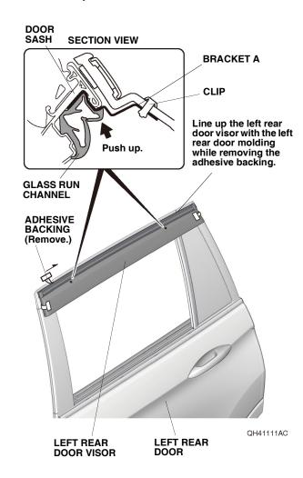
25. Using a rubber roller, apply firm pressure against the left rear door visor and roll from one end to the other. NOTE: Apply firm pressure, especially at the ends.
