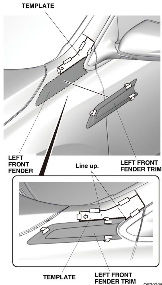
5. While applying light pressure against the left front fender trim, carefully remove the taped adhesive backings.
