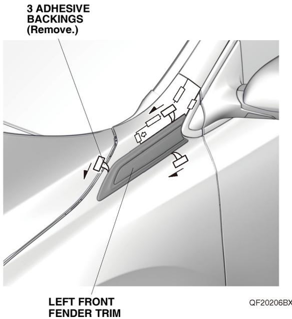
6. Using a rubber roller, apply firm pressure against the left front fender trim and roll from one end to the other. Apply firm pressure, especially at the ends.
