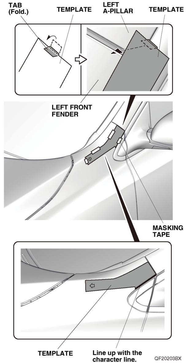
3. Peel back the adhesive backings, and tape them to the front surface of the left front fender trim with masking tape. Remove the remaining adhesive backings.
