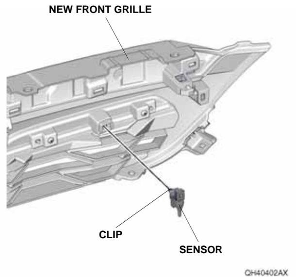
13. Install the new front grille to the front bumper with the eight retaining tabs and two clips.
