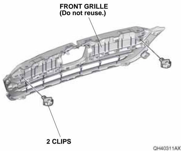
11. Install the two clips to the new front grille.
